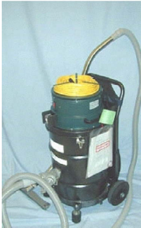
Figure 593-9-7 Vacuum Sanding System
